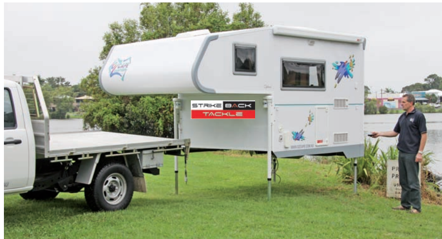
Each leg of the camper can be adjusted, enabling it to sit level on uneven ground.
