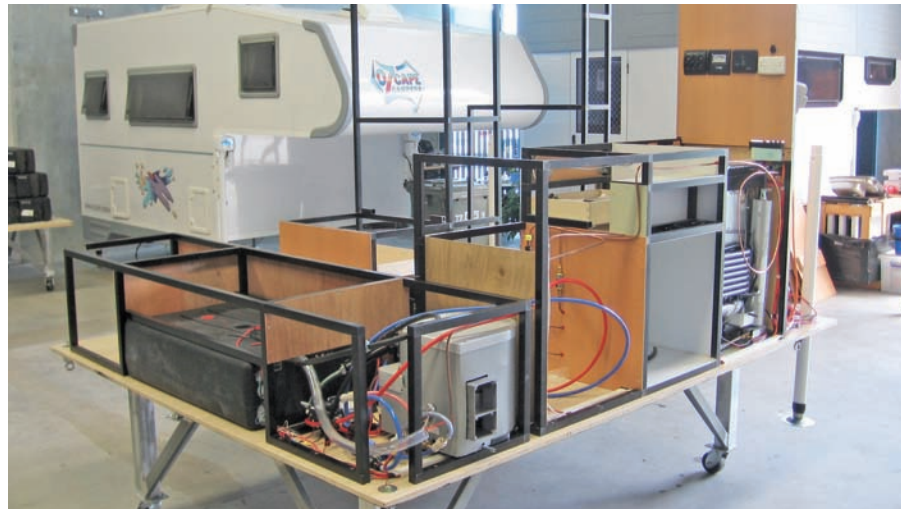
The strength of the unit is maximised and the building process simplified, by constructing the internal fittings on the camper base before the exterior walls are attached.
